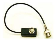
For single (field installed) protection. Designed for today's sensitive cameras requiring inline installation where an independent ground is not an option. Clamps at 11 volts (center pin to shield) and built into a durable weatherproof enclosure. Protects both differential and common modes, enabling ground isolation from shield.
