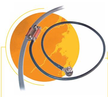
The grounding kit provides a correct electrical contact between the coaxial cable outer conductor and the grounded structure, facilitating the flow of electrostatic or lightning disturbances, and avoiding by this way destructive sparkovers.
