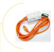
Designed to protect Category 5E/6 data and communication lines running at 100Base-T transmission speeds. All eight pins are protected by a carefully designed circuit for high speed ethernet lines. The ultra-sharp clamping response of the CITEL model MJ8-CAT6 permanently eliminates transients from your local and wide area network applications.
