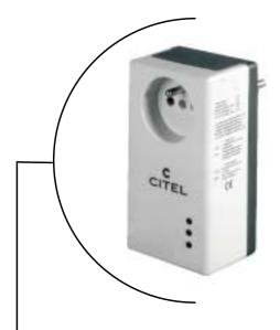
The VM230F protects equipment connected to the single-phase power network from damage by lasting under and overvoltages (several seconds) caused by distribution network fluctuations, short-circuits between networks, connection errors, and neutral disconnection. The VM230F also protects against voltage surges (lightning).
